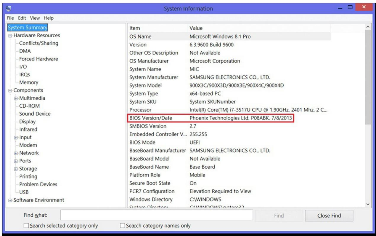
As can be seen in the above screenshot, BIOS info is given under System Summary. BIOS has a Setup utility stored in the BIOS flash memory. The configured data is provided with context-sensitive Help and is stored in the system's battery-backed CMOS RAM. To get into the BIOS on your Windows computer you need to press F2 just after you turn on the computer. A typical BIOS snap shot is shown below:
