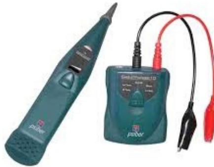
**4. Cable Tester :** A cable tester is used to verify that all of the intended connections exist and that there are no unintended connections in the cable being tested. When an intended connection is missing it is said to be "open". When an unintended connection exists it is said to be a "short" (as in short circuit). If a connection "goes to the wrong place" it is said to be "miswired" (the connection has two faults: it is open to the correct contact and shorted to an incorrect contact).
