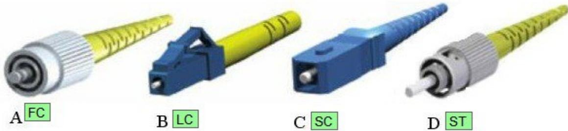
4. **LC cables latch:** LC cables latch release into their jacks in a manner similar to Ethernet connectors. Smaller in form than SC connectors, their durability is not compromised, nor is cost increased. Instead of snapping or thermo forming the connector to the cable, it is glued. This makes it a popular connector for field use.
